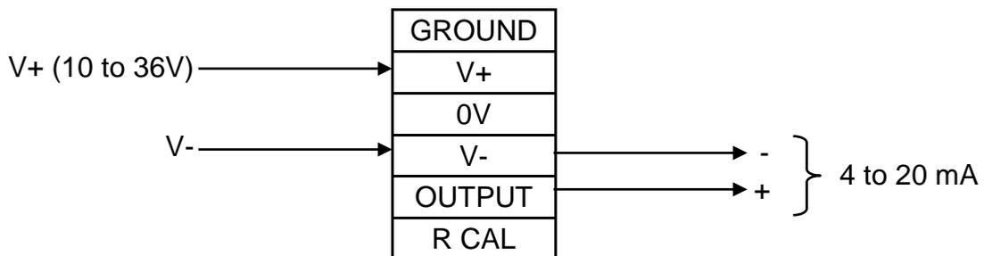
Note 1 Ground is connected to the case of the amplifier.
