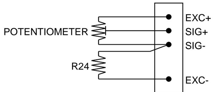
Input signal =  $10 - 1.7 = 8.3V$  so use the lowest gain range for  $\pm 10V$  output. For lower output voltage or 4-20mA output, use lower excitation, e.g. 5V.
